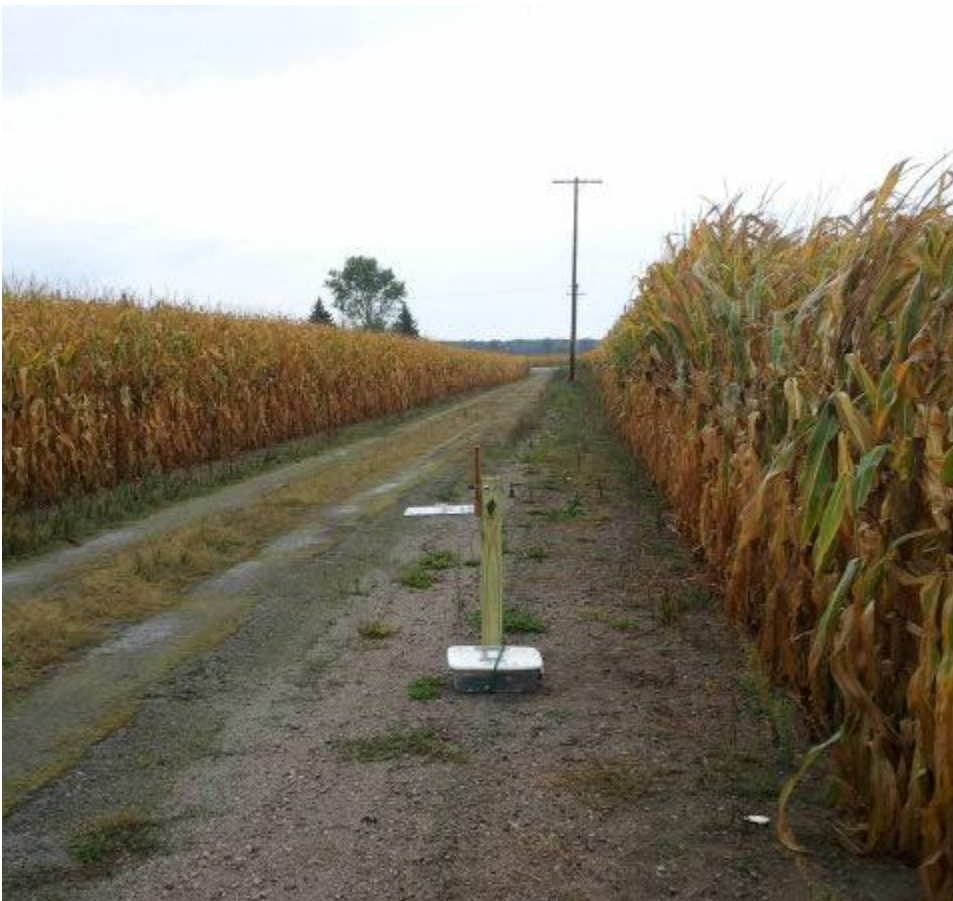
Figure 4. Acoustical monitoring equipment was placed under towers to detect the frequency of bird detections during the fall 2012 migration in order to compare the relationships between avian night flight call frequencies (i.e., attraction) and tower support systems, as well as to compare avian carcass counts under a tower to the number of avian night flight calls.
